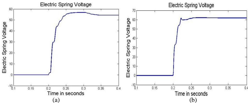
Figure 9. Electric Spring voltage during (a) under voltage conditions (b) over voltage condition
