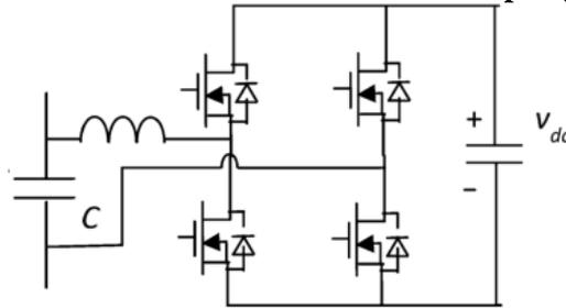
Figure 3. Full H bridge inverter employed in the scheme
