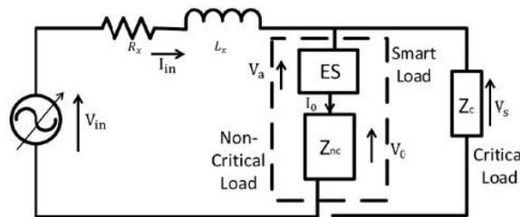
Figure 1. Overview of electric spring in series with noncritical load
