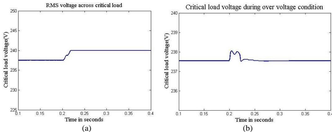
Figure 7. Critical load voltage during over voltage conditions (a) without electric spring (b) with electric spring
