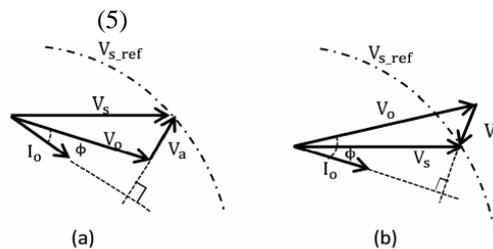
Figure 2. Phasor diagram of Electric Spring (a) inductive mode (b) capacitive mode
