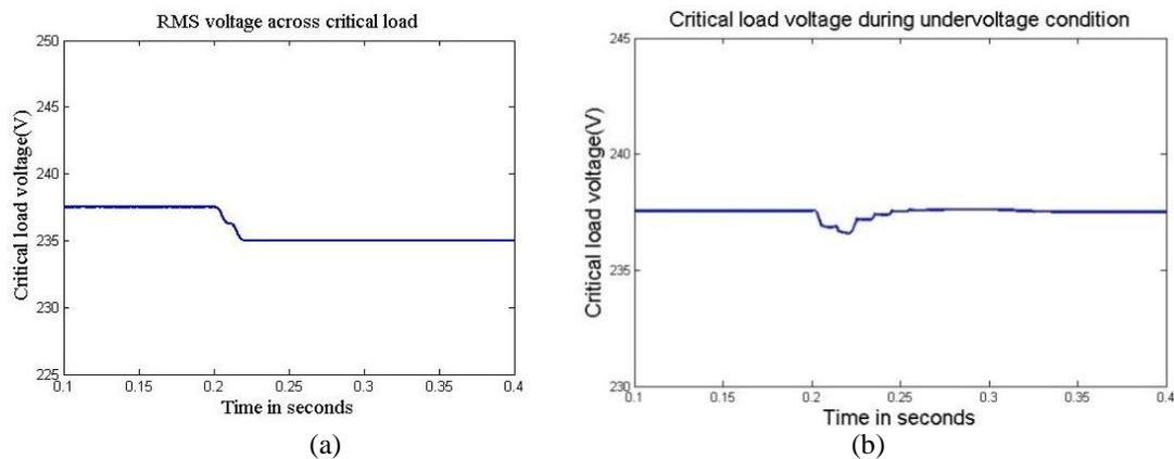
Figure 6. Critical load voltage during under voltage conditions (a) without electric spring (b) with electric spring
