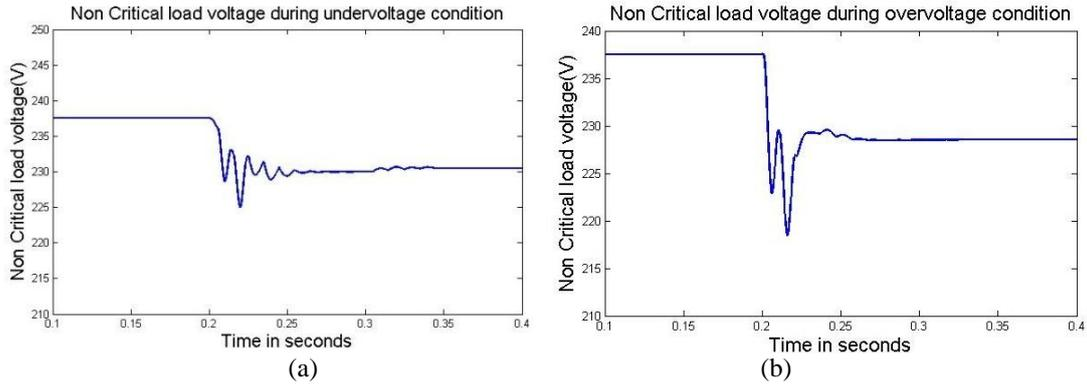
Figure 8. Noncritical load voltage during (a) under voltage conditions (b) over voltage conditions
