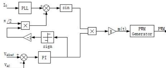
Figure 4. Control blocks of electric spring
